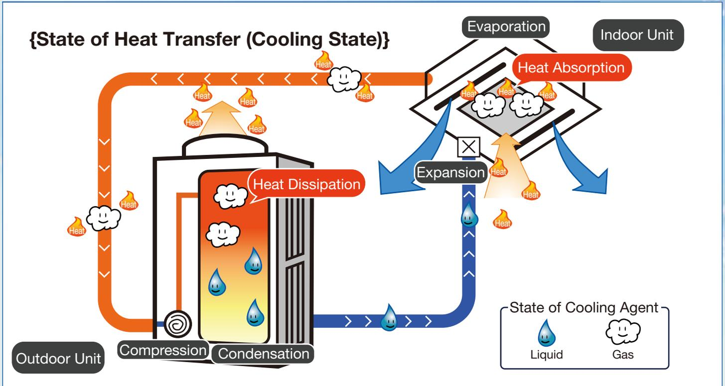
**Incomplete liquefaction of cooling refrigerant causes insufficient heat transfer during evaporation. As a result, an inefficient operation takes place, causing higher electrical bill.**
