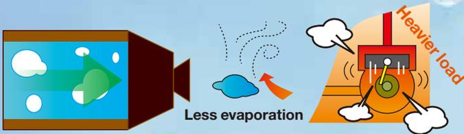
Heat transfer gets deteriorated, hence the compressor load increase in the system causing increase of electric power requirement.
