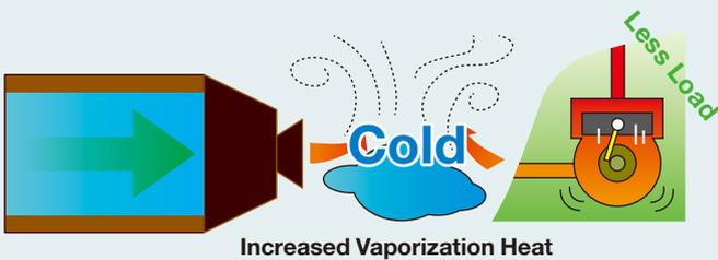
Liquefaction is accelerated with  $\alpha$ -HT's agitation function, leading reduction of compressor load which in turn reduces electric power consumption.
