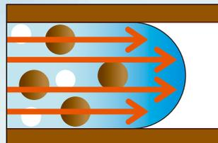
Viscosity of refrigerant becomes resistance which pushes up compressor's load
